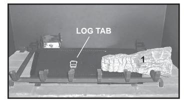
**STEP 2:** Log #1 (SRV2057-720): Place log 1 so that the bottom right notch on log rests on far right grate tine. The bottom left notch on log #1 must mate over the log tab on the burner face.
